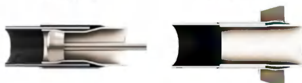
Swaging along the inner surface
